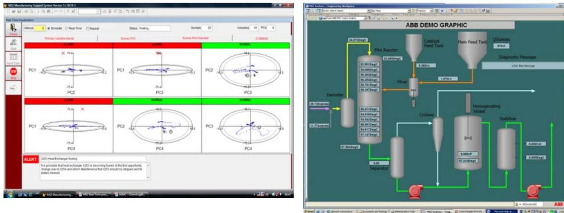
*MS2 (shown on the left) performs the multivariate analysis and sends its results, together with appropriate operator advice, to the ABB System 800xA (shown on the right).*
