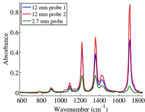
Figure 2: Overlaid plot of acetone analysed using a selection of probes.
