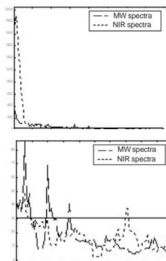
**Figure 3:** Comparison of Caterpillar results to determine end-point of an esterification reaction. The dotted line indicates the NIR spectra and the dashed line the MW spectra. a) the entire reaction, b) smaller part of the reaction to show when the reaction reaches end-point.
