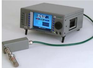
The company has also recently in 2004 introduced a new range of probes that are more suited to both development and industrial bioreactors using bacteria or filamentous cells. A 4 channel version of the Biomass Monitor is also manufactured within an IP65 enclosure and is ideal for production plants.
