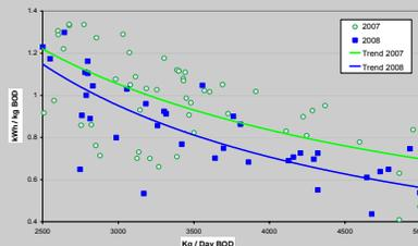
Figure 3: The new control system has been in place for most of 2008. Compared with energy requirements in 2007 under varying process loads, the new control system has reduced energy variability, and driven down average energy consumption.
