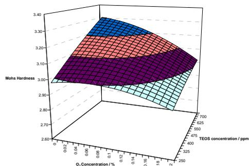
The figure shows the response surface for film hardness as a function of O<sub>2</sub> concentration and precursor concentration.
