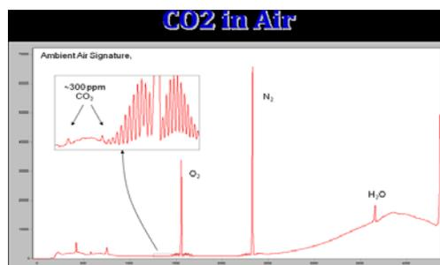
Figure 4: Raman spectrum showing 300 ppm  $\text{CO}_2$  in ambient air. (Image courtesy of Kaiser Optical Systems)
