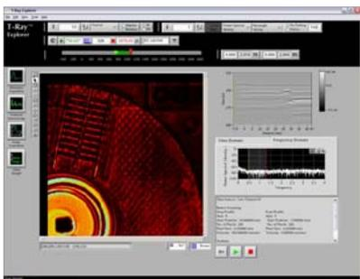
Figure 1: Terahertz image of a floppy disk showing detail through the plastic cover (Image courtesy of Picometrix Inc.)
